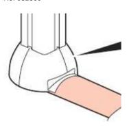
A mini-column can be connected to a floor duct Cat. No. 032800.
